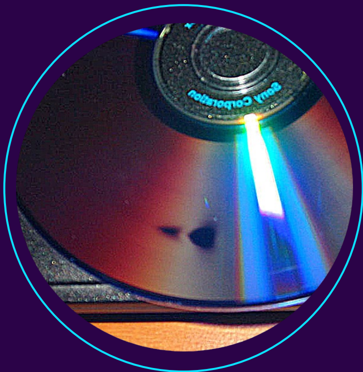
An example of “disc rot” in which the aluminum layers of a disc begin to oxidize.
